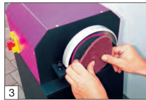
3 Uses the FIX HOOK AND LOOP SYSTEM (See pages 23-25). For replacement flap discs, see page 13.
